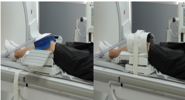
Figure 2. The image on the left shows the placement of the passive driver and the gel pad. The picture on the right shows the passive driver and gel pad inserted into the coil, and the coil in the closed state.
